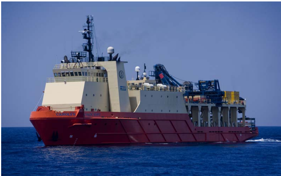
View from Port side showing node handling deck and top ROV deck
