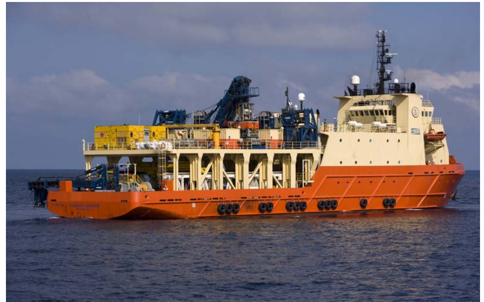
View from Starboard side showing node handling deck (mid) and top ROV deck
